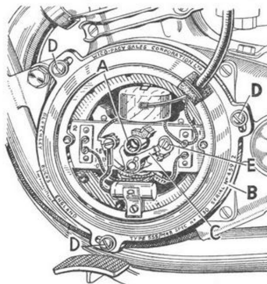
Fig. D4—The Contact Breaker Mechanism.
