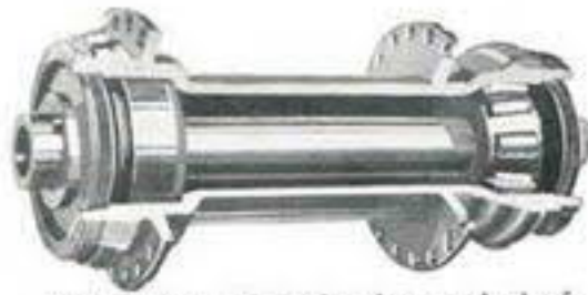
Timken Rear Hub showing method of sealing to retain lubricant and exclude dirt and water.
