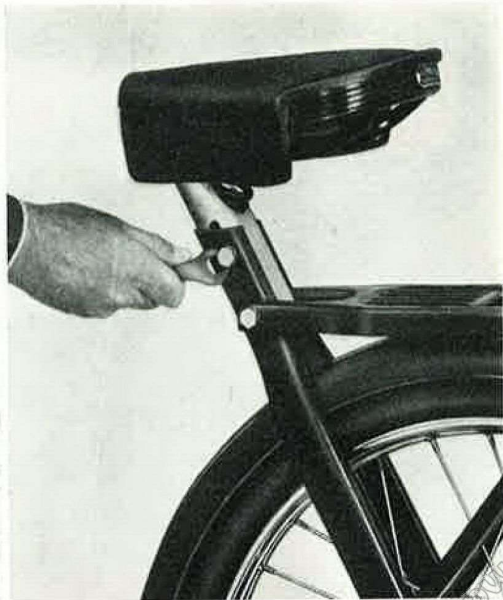
Fig. 13 - Setting the position of the saddle.
