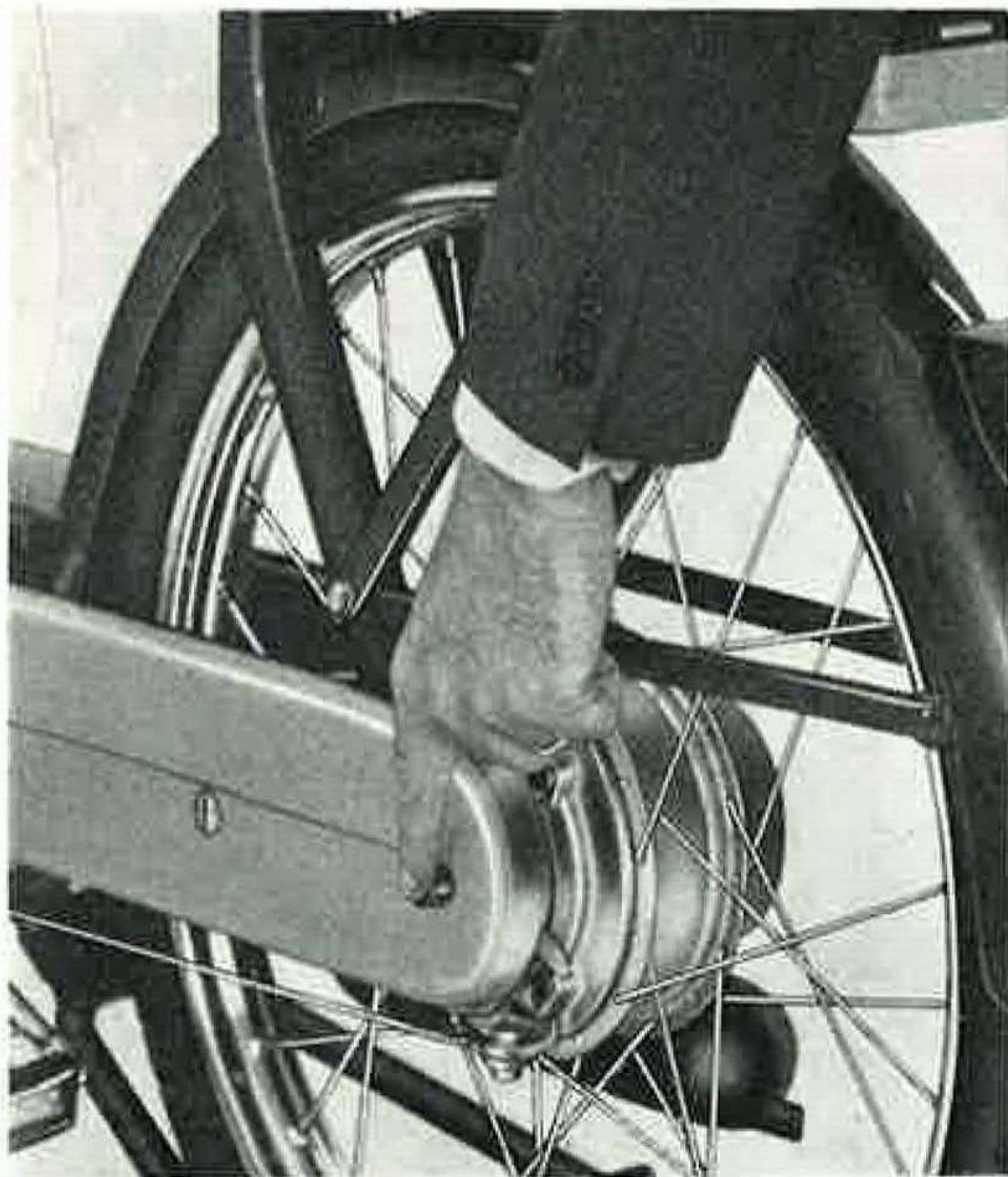
Fig. 5 - Acting on the disconnecting knob of the rear wheel from the engine.
