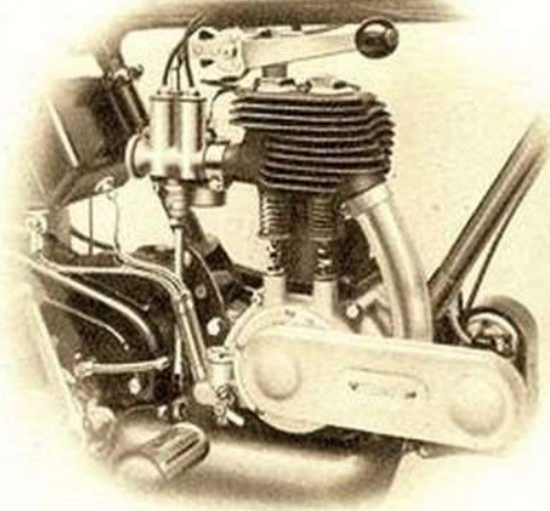
The power unit of the 4.94 h.p. Model N.L.
