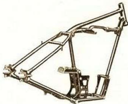
The straight tube cradle frame of Models C.N., C.O., and C.S.D.
