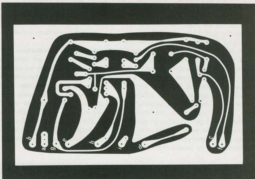
Fig. 6. Etching and drilling guide for the Siren Driver module's printed circuit board is shown above. Artwork for this and the other two pc boards on this page appears full-size.
