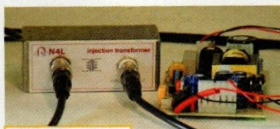
Figure 2 An injection transformer injects a disturbance signal into the control loop of an open-frame switched-mode power supply. At each injected frequency point, measure the relative amplitude in decibels and the relative phase in degrees.
