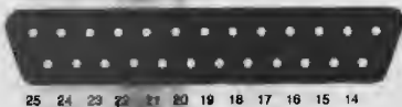
(a) Pin-out of the Centronics connector on pc compatibles - viewed from the back of the pc Connector type: 25-pin female D-type
