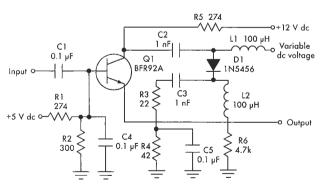
The variable dc voltage applied to this circuit changes the diode's capacitance in a predictable way. Thus, the phase of the output voltage can be controlled.
