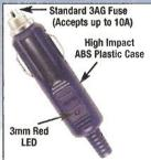
accepts a standard 3AG fuse and is supplied with a 250 volt 3 amp type. An optional 3mm red LED (when lit) assures that the unit is receiving power. The plug unscrews for easy soldering.
