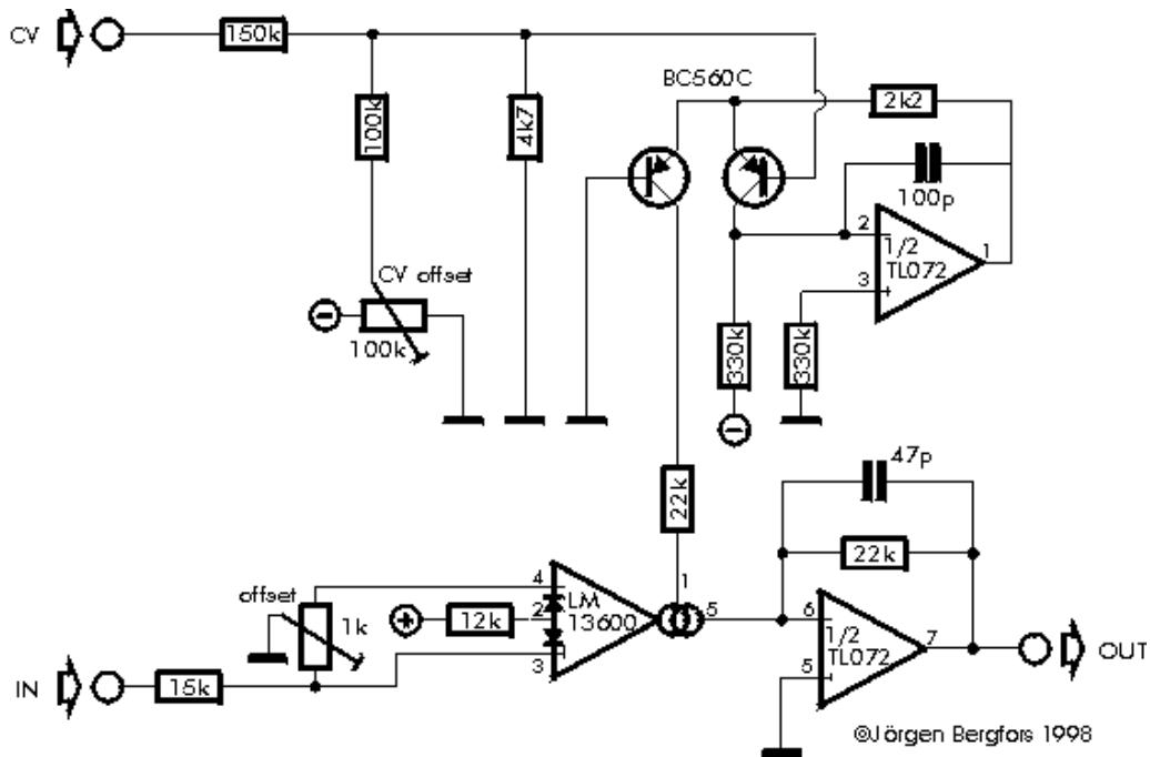
This circuit is identical to LM13600 VCA 1, with the exception of the output stage. Here, the load resistor is in the feedback loop of an inverting amplifier, instead of connected to ground. The effect this has on performance turned out to be negligible. Signal bleedthrough seems to be very slightly better, which makes this circuit the overall winner.
