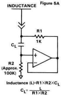
The National Semiconductor Audio/Radio Handbook recommends a Q of 1.7 for an octave equalizer described in its pages, though the Q must of course be higher for a third-octave unit. You probably don't want the Q to ever exceed 4 or 5, to minimize phase shift and ringing. The trade-off in the other direction (lower Q) is less control, since the filters will interact creating bumps in the response when adjacent bands are boosted or cut.
