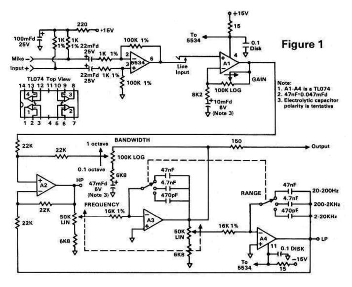
The circuit shown in Figure 1 uses only two ICs, and has a bandwidth that is adjustable from more than one octave down to a tenth of an octave. As shown, the frequency range is 20 Hz. to 20 KHz. in three bands, although a fourth subsonic band could be added to allow very low frequency analysis. A low-noise mike preamplifier is included, and a line input is also available with up to 20 dB of gain. Of course, you could use a mike preamp in your console instead, but at the expense of portability.
