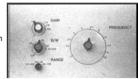
standard third-octave frequencies from 200 Hz. to 2 KHz. These same marks will serve to identify the proper points on the other ranges as well.
