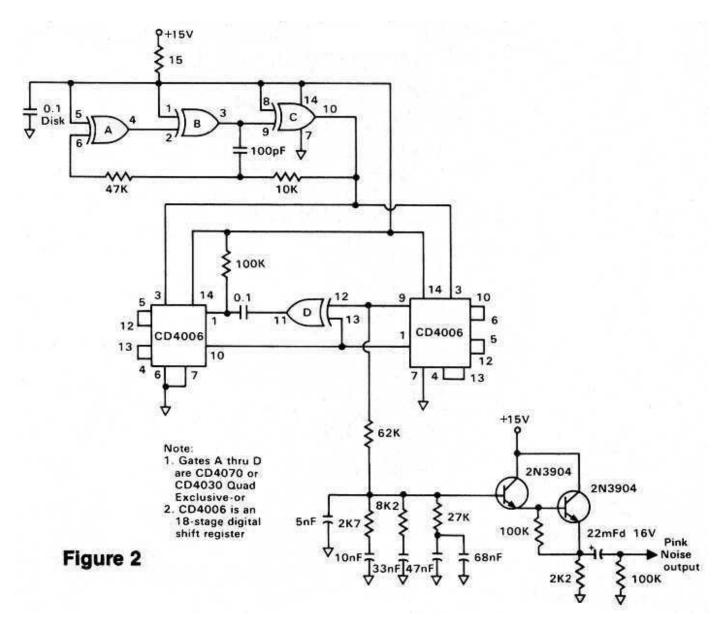
Pink noise - which contains all frequencies simultaneously - is frequently used as a signal source when measuring speakers. Many noise generator designs use a reverse biased semiconductor junction as the actual noise source. But this requires you to test many transistors, select one that
