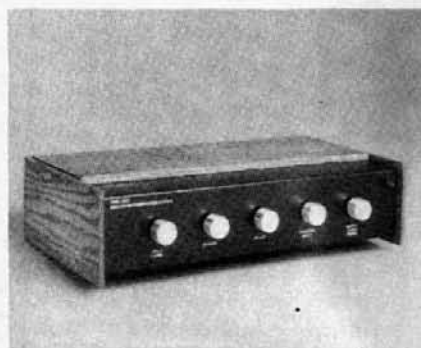
FIG. 11—THE COMPLETED REVERB unit. Enclosure shown is included with kit available from supplier listed in Parts List.
