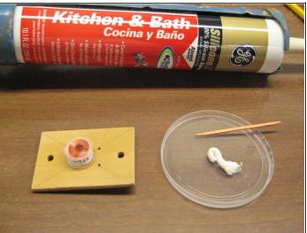
• To mount the pickups for wiring, I drilled 2 small holes in a piece of very thin plywood, inserted 2 brass escutcheon pins on the underside of the plywood to use as soldering posts, passed the magnet wire leads through the holes, and mounted the bobbin using a dab of hot glue or silicone caulk.
