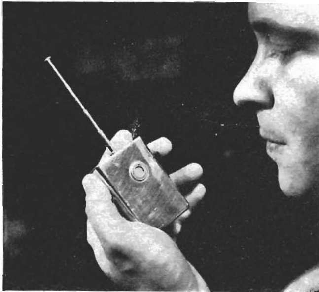
Fig. 1. Miniature transistorized FM transmitter shown in use.
