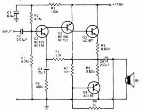
A high input impedance of 1.1 megohm is made possible in this amplifier by keeping the collector current of Q1 low, and by using a high level of ac and dc feedback. The input sensitivity is adjusted by altering the value of R3.
