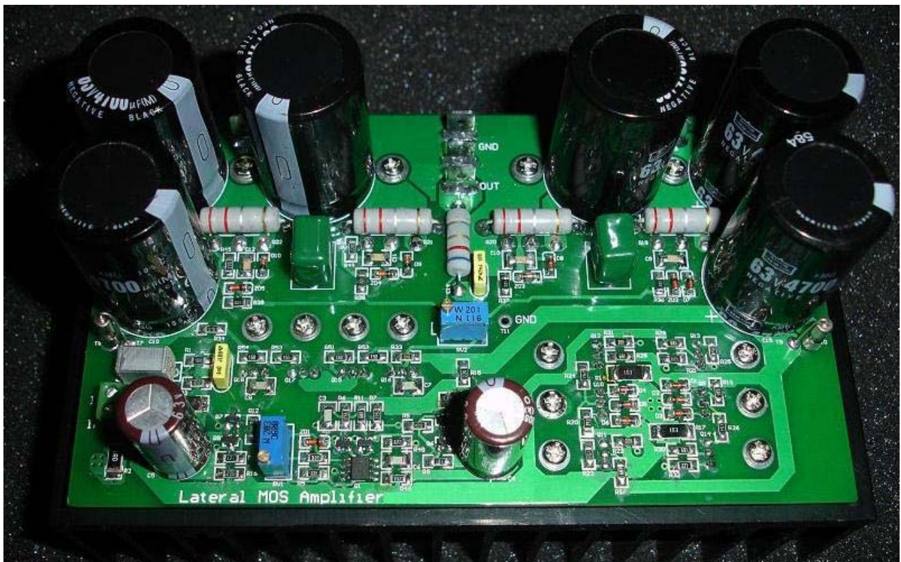
Figure1: Complete assembled AEM6000 Audio Amplifier and mounted on the heatsink.
