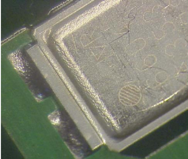
Figure 3 External solder fillets on the drain
