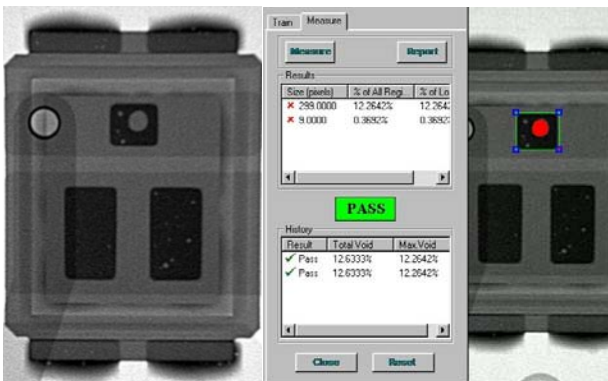
Figure 12 Voids on the gate contact
