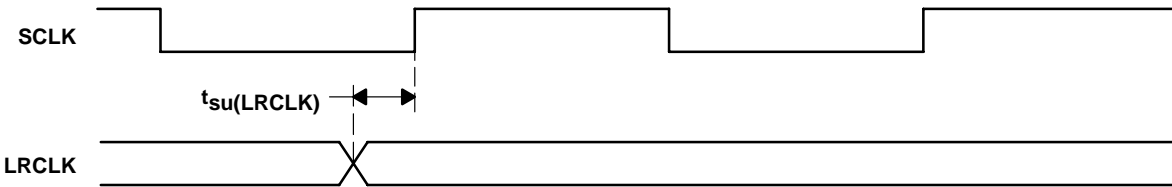
Figure 12. Right, Left, and IIS Serial Mode Timing Requirement
