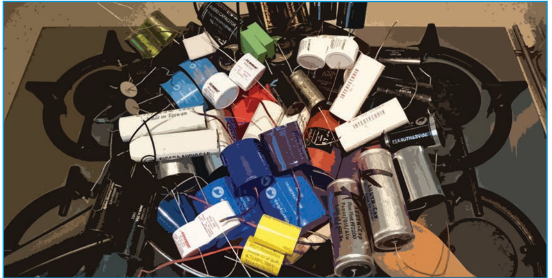
Photo 2: Mechanical resonance is a key feature in audio capacitors, which come in a variety of types and sizes. (Photo courtesy of Humble Homemade Hifi, www.humblehomemadehifi.com/Cap.html )
