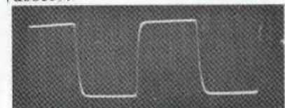
10 KC square wave from Dynakit (below) is much like original (above).
