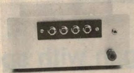
Back panel view of the unit. The two output sockets are at left while the input sockets are at right.
