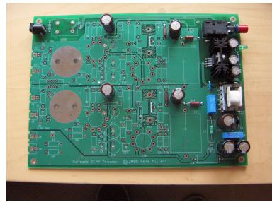
The big round shiny circles are spots for <u>Sowter</u> moving-coil step-up transformers. The power transformer can be seen near the right-hand edge. The heatsinks that are not installed are for the IXCP10M45S CCS parts.
