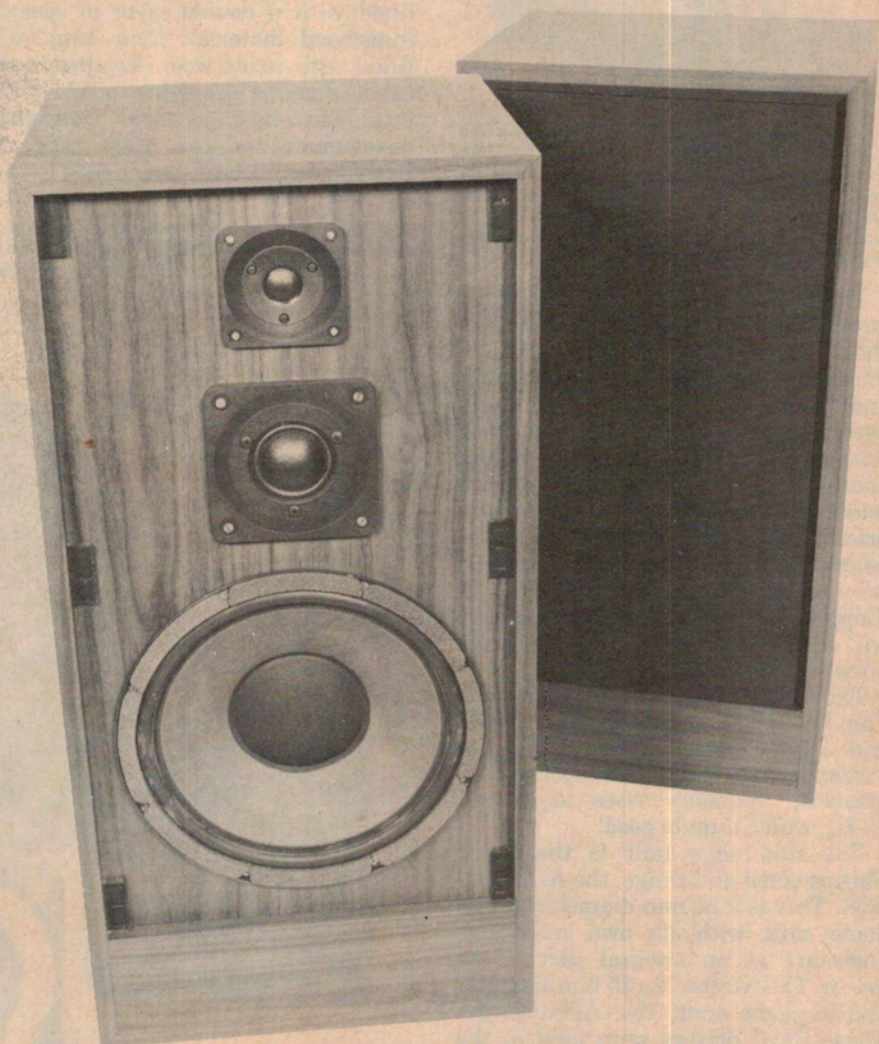
► View of the completed speakers, with and without the front grille. We secured the latter to the front baffle using Velcro strips stapled in appropriate positions.
