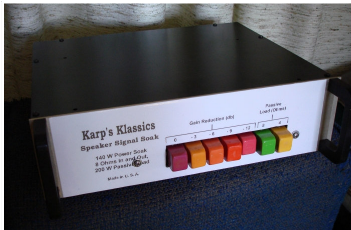
Figure 3 - My amplifier output attenuator box
