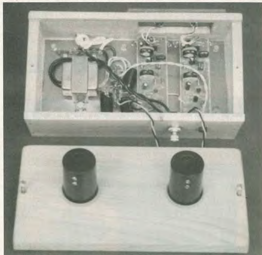
FIG. 7—MOUNT THE MODULES for the stereo transmitter in a cabinet along with the power-supply components or a battery pack if you so desire.
