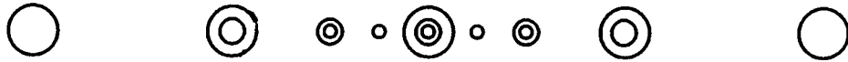
FIGURE 19.2 Three superimposed linear arrays depicted by large, midsize, and small circles. The largest array covers the low frequencies, the midsize array covers the midrange frequencies, and the smallest covers the high frequencies.
