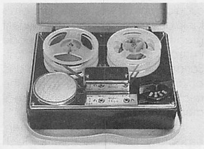
Fig. 10. Acme Model 1500 recorder. A modest 3-inch reel machine, using "rim drive" and a swing-out permanent magnet to erase previous recordings when in the record mode.
