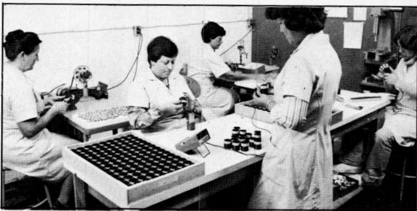
Voice-coil assembly at Sound Dynamics factory in Markham, Ontario
