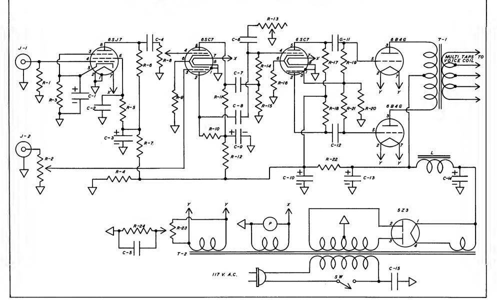
This is a 10 watt high-fidelity amplifier which is designed to operate from a high impedance microphone and phonograph pickup simultaneously. A phase inverter tube is used to provide push-pull operation to the power output tubes. The output tubes can be either 6A3 or 6B4G types for six volt operation, or 2A3 tubes if  $2\frac{1}{2}$  volts is available for filament operation. A hum balancing control, R-24, can be adjusted to balance out any hum present in the speaker.
