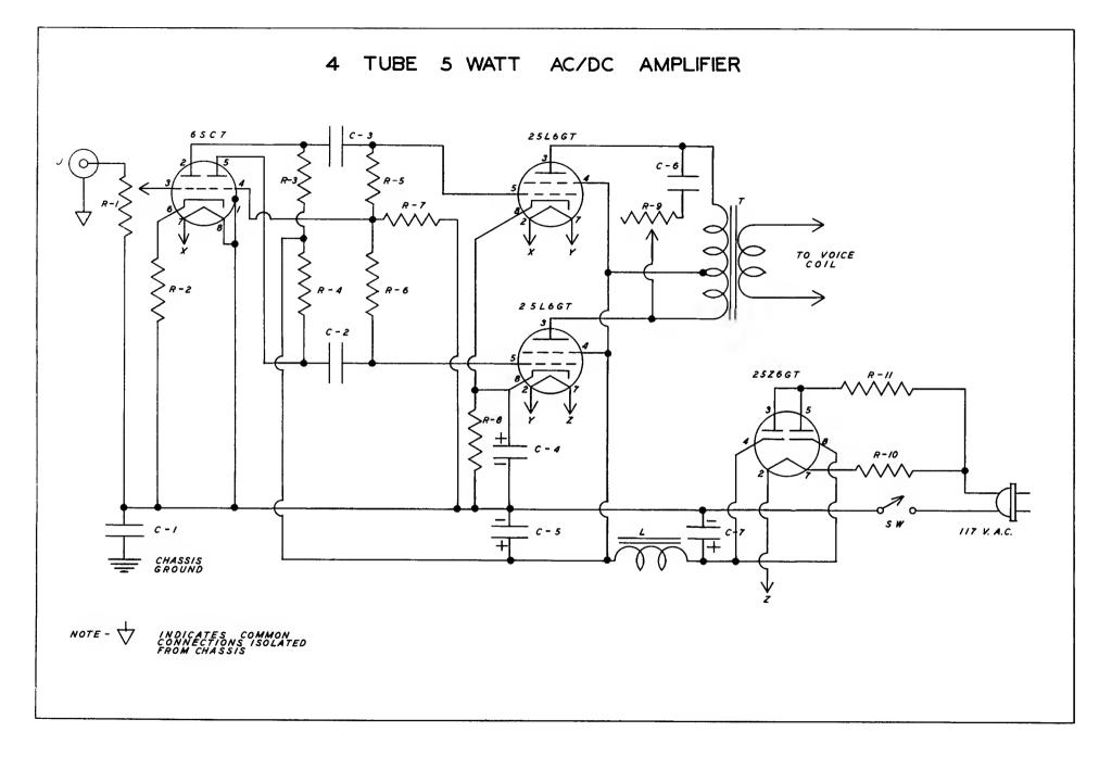
The amplifier shown is of the push-pull type, suitable for operation from a phonograph pickup or radio tuner. It is capable of good room volume and fine tone quality due largely to its power output circuit. Having a"transformerless" AC/DC rectifier, the amplifier can be built very compactly, making it ideal for portable purposes. It also operates from either 110 volts A.C. or D.C.
