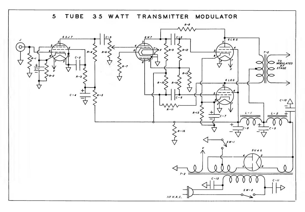
This 35 watt amplifier is quite suitable for modulating an amateur or commercial 50 to 75 watt transmitter. It is designed for a single crystal or dynamic microphone input and has considerable over-all gain. A 6SJ7 high gain stage operates into a 6N7 phase inverter, and thence into the push-pull 6L6G tubes for high power. A load should always be applied to the output transformer secondary to protect it against accidental burnout.
