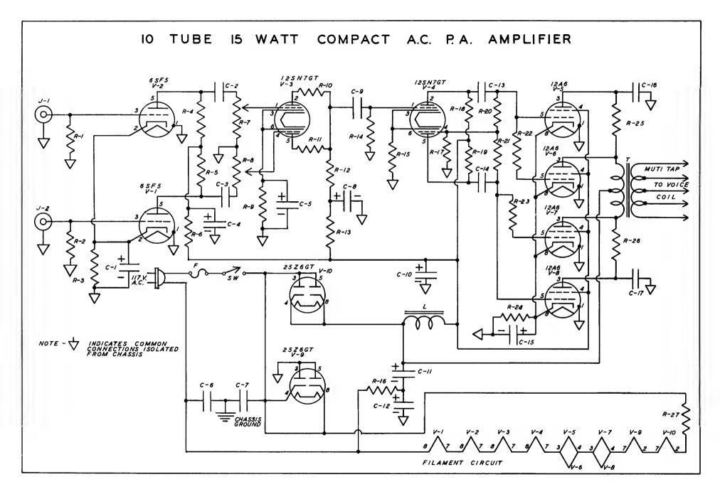
Here is a special "transformerless" amplifier having a series filament circuit and a voltage doubler rectifier capable of 15 watts output. It has sufficient gain for high impedance microphone operation, and is designed to handle two of them through an electronic mixing circuit. A low level phonograph pickup may be used in one channel if desired.
