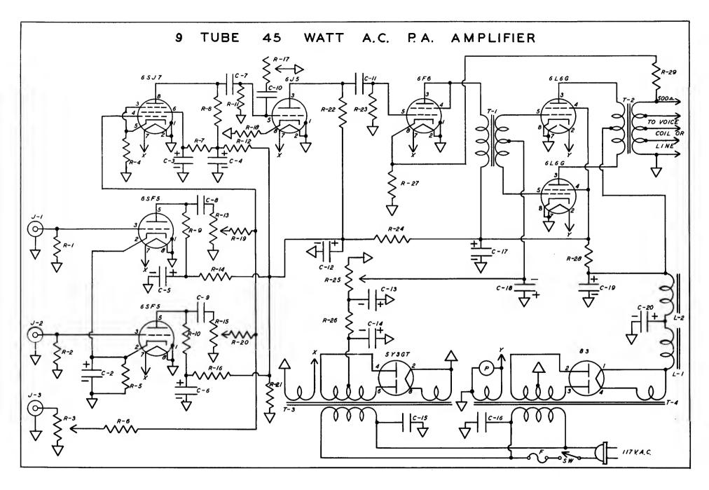
A 45 watt public address amplifier is shown having two microphone and one phonograph inputs. The amplifier uses fixed bias in its output circuit for greater power, and R-25 is pre-adjusted for  $-22\frac{1}{2}$  volts bias on the 6L6G tubes. An inverse feedback network consisting of R-29 is incorporated for improved tone quality.
