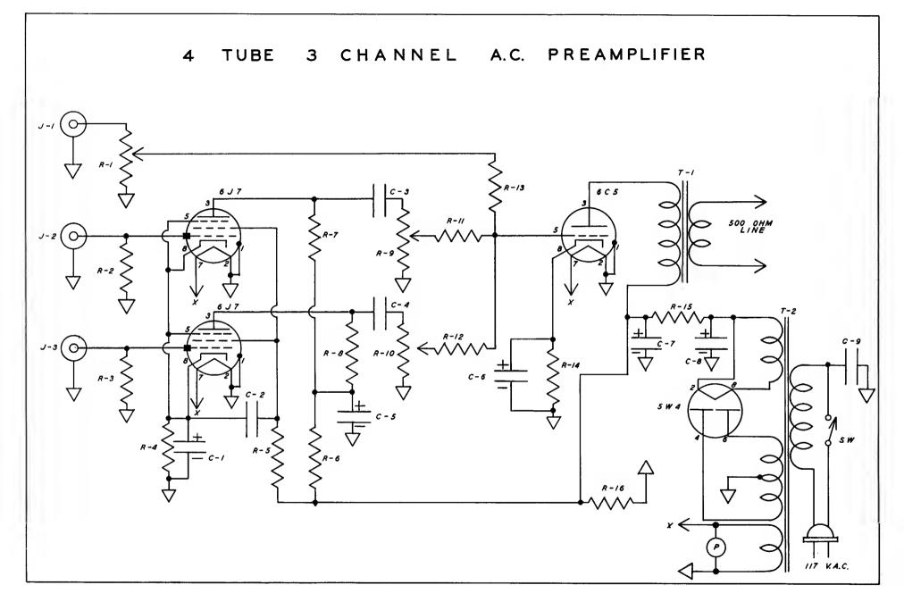
A normally low gain amplifier can be operated from a preamplifier similar to the one shown. This designed for a phonograph pickup and two high impedance microphone inputs. These three inputs can be mixed at will to feed the output circuit to the 500 ohm line. Of course, the amplifier following this preamplifier must have an input transformer designed for 500 ohms input.
