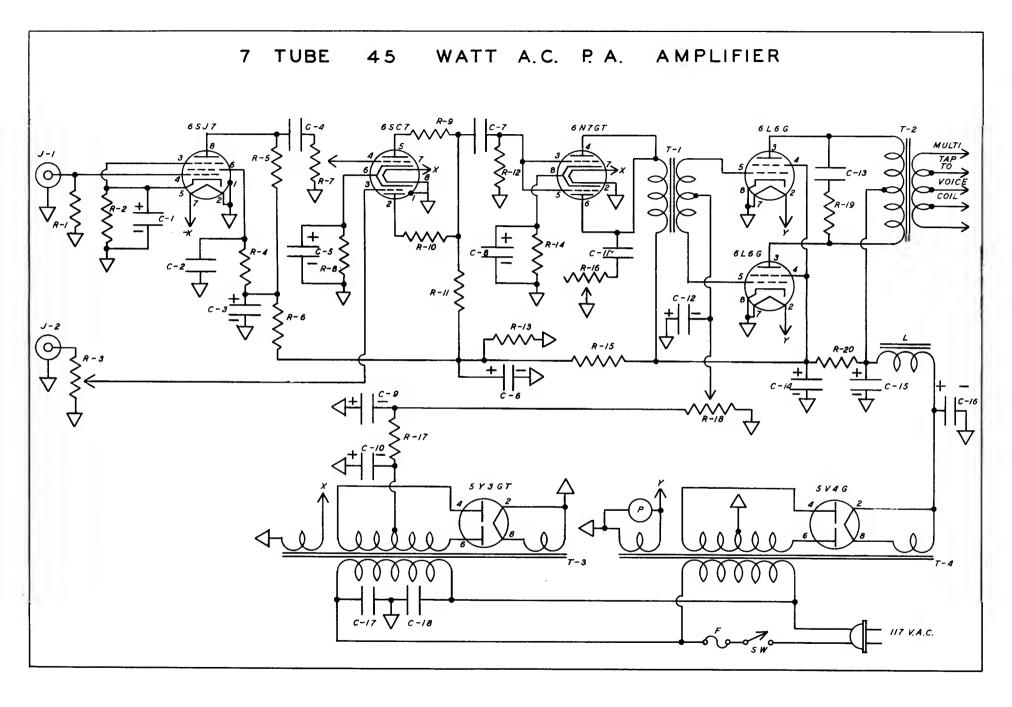
A high power output public address amplifier utilizing push-pull 6L6G tubes is shown. Fixed bias and sufficient driving power for the output tubes provides this high power to the speakers. Voltage dividing resistor (R-18) is adjusted for  $-22\frac{1}{2}$  volts on the tap. A high impedance microphone and phonograph pickup may be used simultaneously and adjusted separately by means of R-7 and R-3; R-16 is a tone control.
