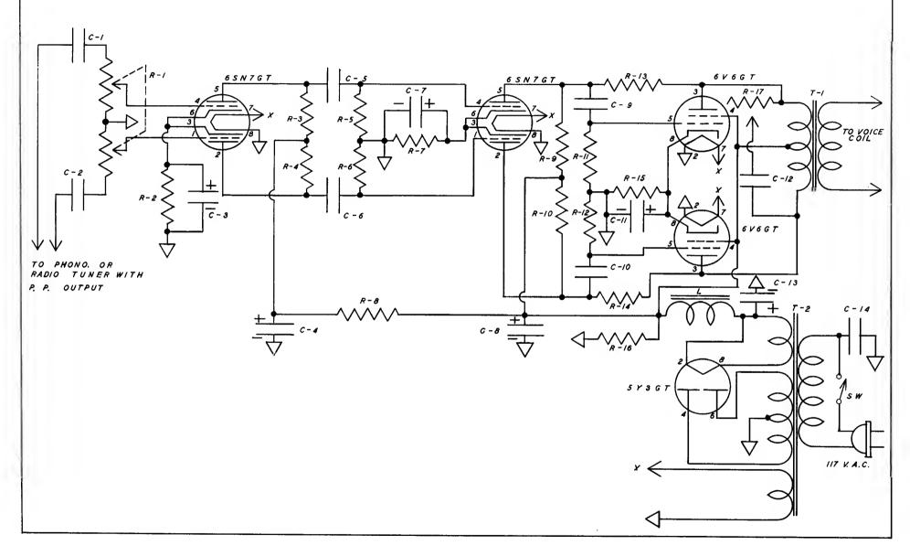
Here is an A.C. amplifier of very fine tone quality, having all push-pull stages. Likewise, it is suitable for operation from either a phonograph pickup or radio tuner. When connected to a crystal pickup unit, the input leads connect directly to the pickup. If a radio tuner is used, a high quality 1:1 ratio input transformer should be used, having a push-pull secondary in order to get proper push-pull input. Inverse feedback is provided through resistors R-14 and R-15.
