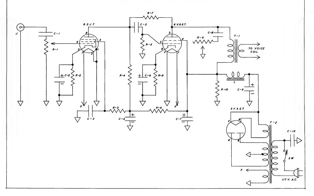
For a small amplifier having good gain and tone, the reliable circuit shown is very satisfactory. It will operate well from either a phonograph pickup or radio tuner and deliver good room volume.
