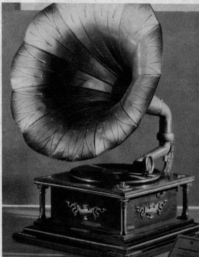
Disc machines, like this early Parlophon, ultimately took over from the original cylinder format. Discs were more economical to produce, as they could be stamped out — a process that hasn't changed in its essentials to this day.
