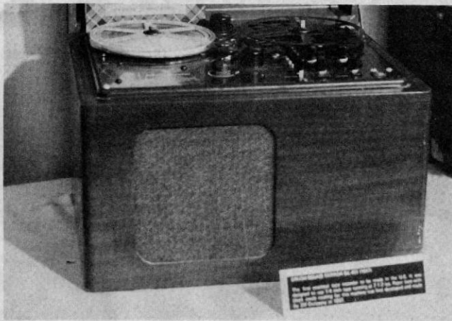
Tape machines for home use followed very quickly, one of the earliest being the Brush "Soundmirror", which used paper tape.
