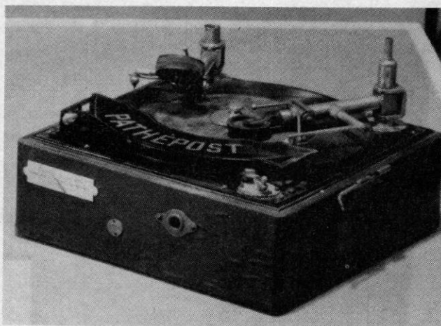
Forerunner of the "tape letter" was this small disc-cutter/reproducer from Pathé in France. Dating from 1910, it is one of the earliest home-recording machines.
