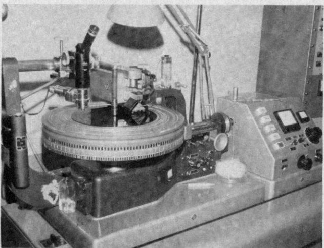
Mastering a modern stereo record, using a sophisticated lathe. In principle, the disc cutting process has not changed since it was developed by Berliner at the beginning of the century.
