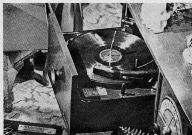
The desire to play pieces of music longer than the four-to-six minutes available on one side of a 78 r.p.m. disc led to the development of record changers, like this familiar Garrard from the 50's.
