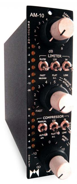
The limiter section is a peak detecting hard-knee style, its control signal being taken from the output of the Effect level pot. Limiting ranges from approximately 25dB down to 4dB. With a little experimentation, many severe and colorful compression effects are possible. This section also includes its own three-position high-pass sidechain filter.
