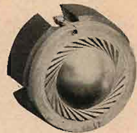
Fig. 3. The high-frequency driver, shown in actual size.
