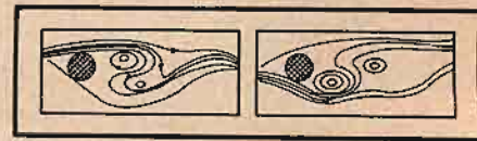
Fig. 4-3. Successive eddies formed by water flowing past an obstacle. (After Sir James Jeans, "Science and Music," The Macmillan Co., 1937.)
