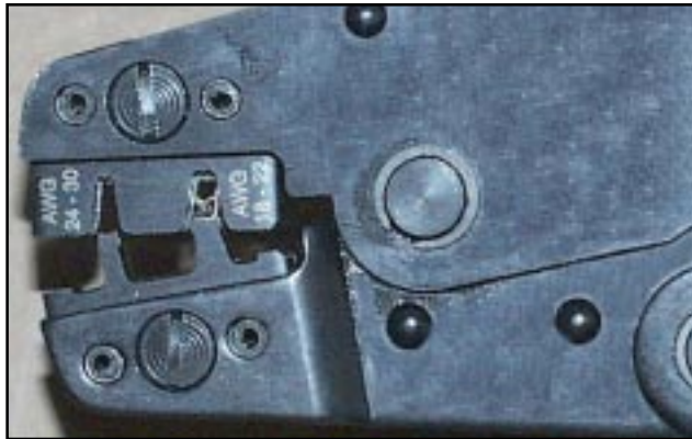
(2) The terminal conductor tabs (pointing UP) are placed in anvil 18-22; the terminal's insulation tabs extend in front towards the camera.
