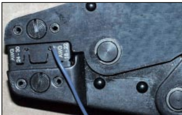
(4) Final step: jaws fully closed; the insulation tabs have been crimped.
