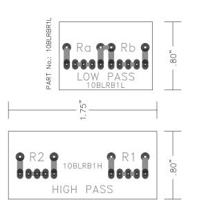
This board is used with the 2nd version of the 10B-LRB. The same board is used in both High Pass and Low Pass filter sections. Two of each board are used in the High Pass filter, and two are used in the Low Pass filter for a total of four boards for each crossover channel, and 8 boards for a two channel 10B-LR crossover.
