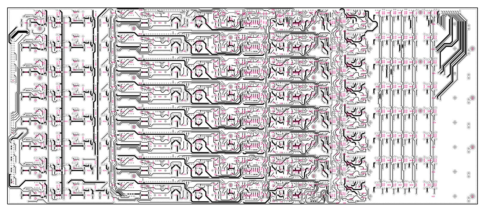
Top (component side) of board Dotted lines are the copper pour layer
