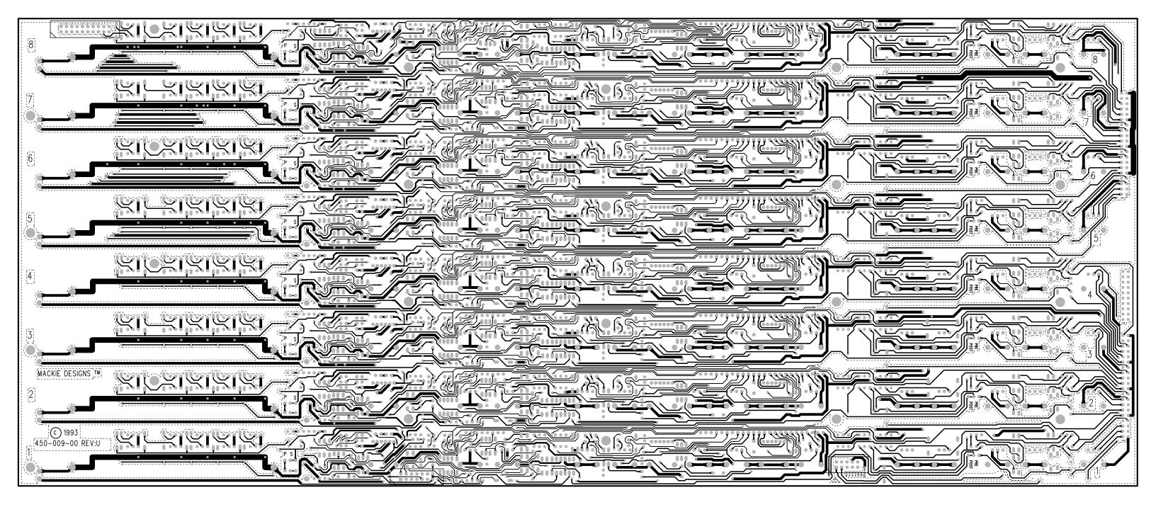
Bottom (solder side) of board Dotted lines are the copper pour layer
