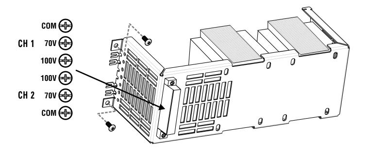
The IT-42 is an output isolation transformer accessory for the QSC CX302 amplifier, allowing it to drive two 25-, 70- and 100-volt distributed lines in stereo or parallel or a single 140- or 200-volt line in bridged mono. The IT-42 is pre wired for quick and convenient mounting to the back of the CX302 amplifier and requires no additional rack space.
