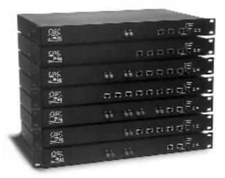
QSC's Audio Transport Hubs, specifically designed for RAVE audio distribution systems, give you the confidence and convenience to create digital networks carrying up to 64 channels of 48 kHz, 20-bit digital audio over standard Fast Ethernet network media. They allow multiple RAVE units to operate together on a network, and several models also convert unshielded twisted pair media (TX) to and from multi-mode optical fiber (FX), for long distance transmission up to 2 kilometers.
