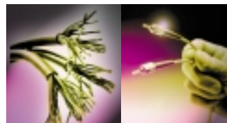
Replace audio cable with a single CAT-5 network cable, or for longer distances (>328 feet or 100m), with fiber optic cables.
