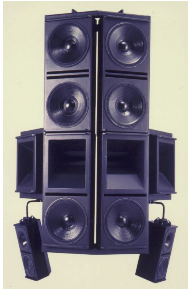
Fig. 11 Reference Point Array using four 40^\circ \times 40^\circ mid-high enclosures and six low frequency modules in Tri-Polar configuration for vertical pattern control, along with appropriate small full range systems for downfill.
