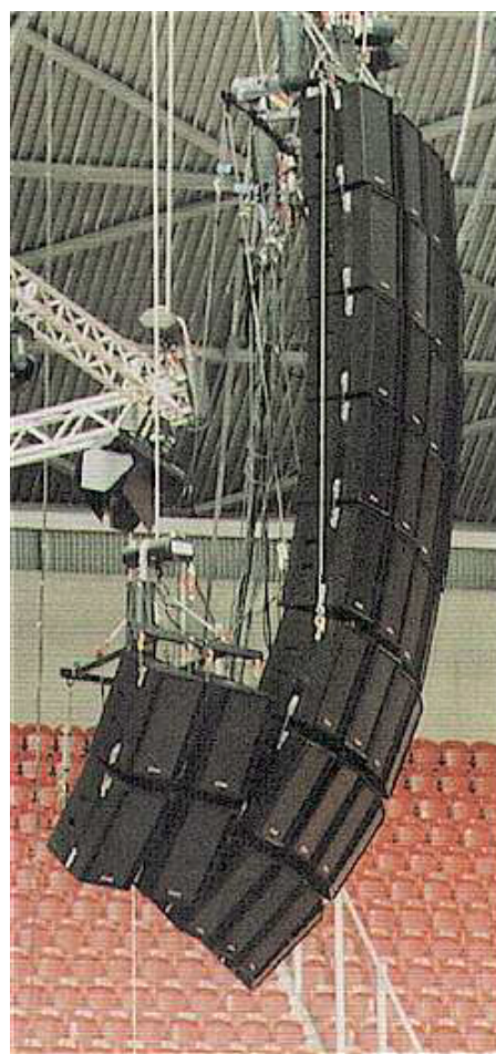
Even when a single enclosure is designed to resemble a point source, multiple enclosures will always interfere with each other when connected to a coherent audio signal.
