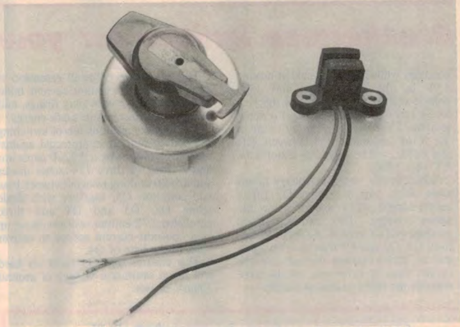
New distributor parts: Bosch rotating vane assembly (left) and Siemens Hall Effect sensor.
