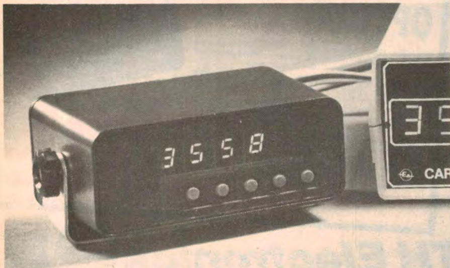
The remote display option is housed in a small plastic case measuring 110 x 70 x 50mm. Unit is compact enough to mount on virtually any dashboard!
