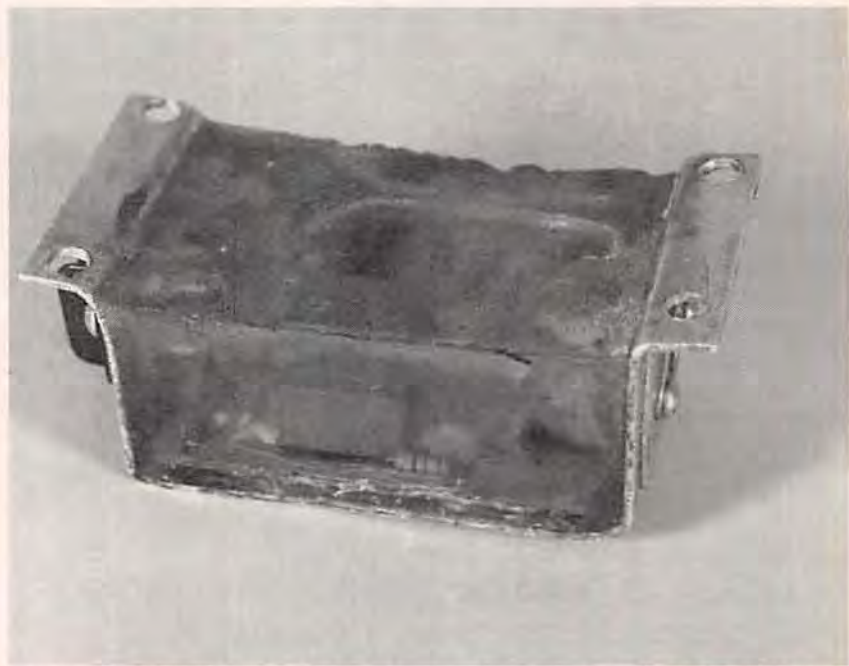
FIG. 6—THE ENTIRE CIRCUIT is encapsulated in a clear plastic resin block help it withstand vibration, humidity, and temperature extremes.
