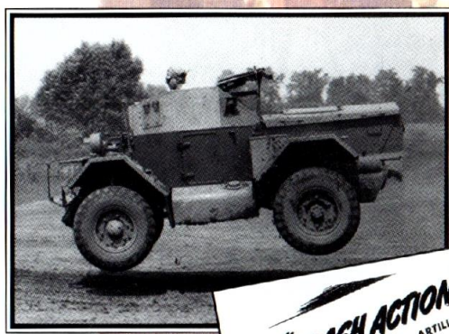
Above: With four wheels off the ground, the Scout car is put through its paces prior to shipment overseas. Scout cars usually underwent 75 miles of rigorous road testing before final inspection.
