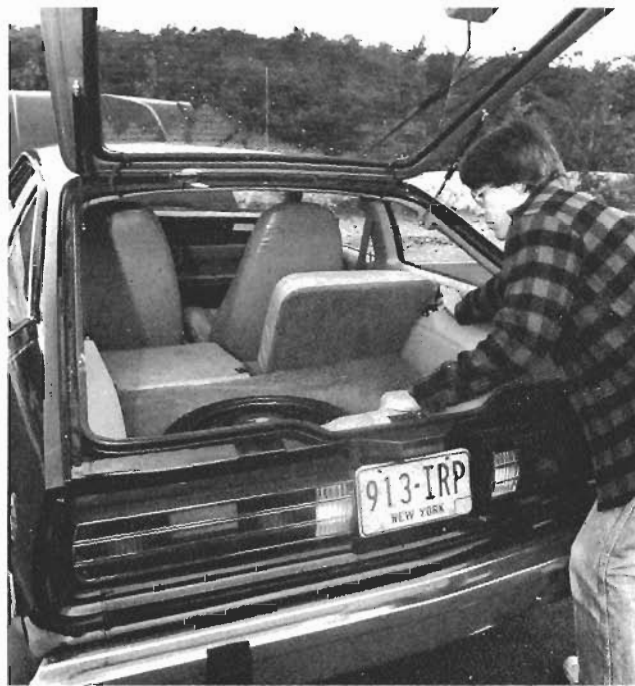
Spirit's large hatch and fold-down split rear seat permit easy carrying of long or bulky cargo, even with one rear passenger.
