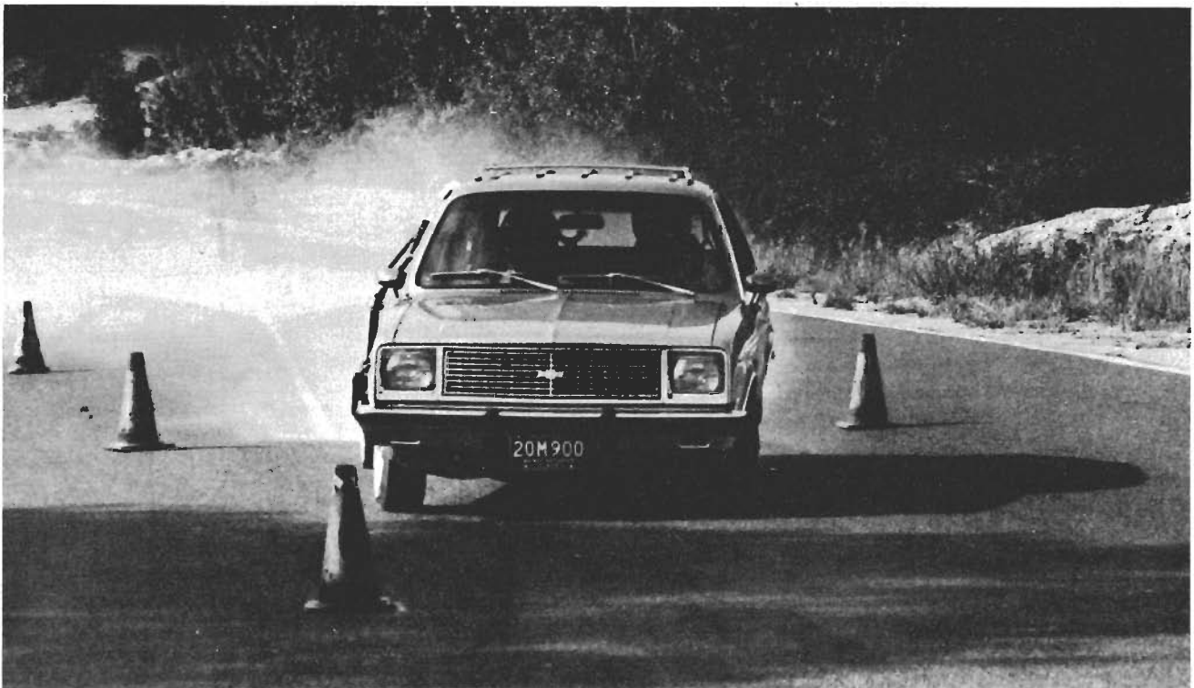
Braking problems plagued both Spirit (above) and Chevette (below). Spirit became unstable during its first 60-mph
