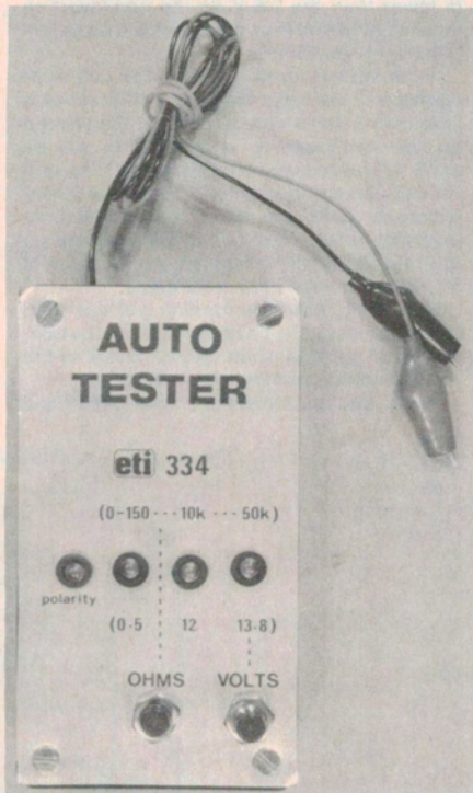
Pragmatic. Simple, but functional. The project was housed in a small jiffy box with a Scotchcal panel added.
