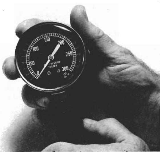
Needle on compression-gauge dial holds at maximum reading. After noting it, press valve to allow needle to drop to zero before you check the next cylinder's compression.
