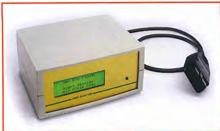
Figure 2. Prototype of the stand-alone OBD analyser.
