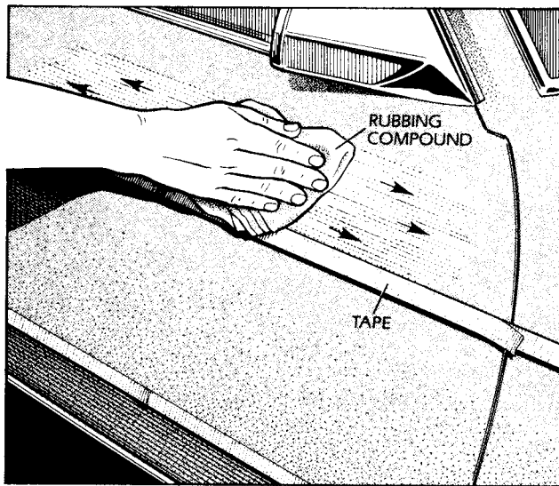
4 Before you compound, use masking tape to protect raised edges.
