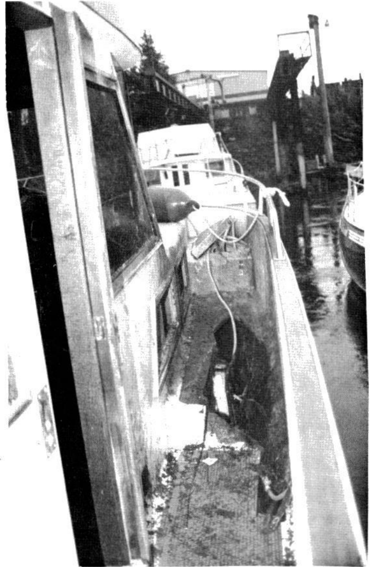
The Tragic result of poor or improperly used wiring.
