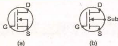
Figure 2. Standard symbols of (a) three-pin and (b) four-pin n-channel enhancement-mode MOSFETs.
