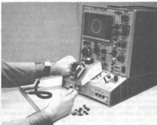
Figure 8b. Curve Tracer. Note wrist strap grounding and Static-Dissipative tabletop surface.
