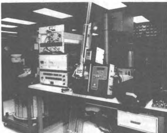
Figure 8a. Automatic Tester for HEXDIPs using Anti-Static Feed and Bin Tubes.
